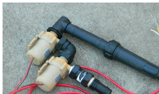
Two pumps connected in series to create a double pump. A filter is connected to the inlet of the first pump.
