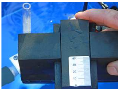
40 mm gap between the bottom of the float and the bottom of the slides
