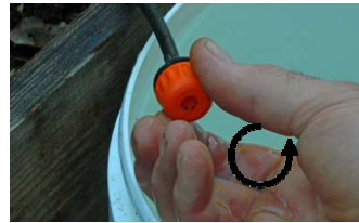
If the volume in the measuring container is more than the dripper control volume, turn the control dripper anticlockwise to increase the flow rate of the control dripper.
