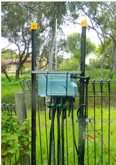
Flow-splitter supplying water to 11 zones. Each outlet valve is adjusted so that the head in the pressure monitor tube for the zone matches the head in the flow-splitter.
