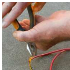
Use pliers to push down the red cap
