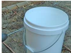
Drill a hole in the side of the evaporator
