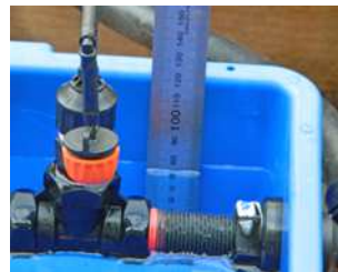
Measuring the depth of water in the evaporator at the low level for UMIC
