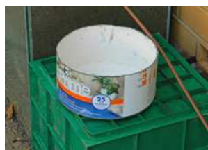
An evaporator with a surface area of 370 square cm
