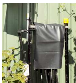
Light-proof cover protecting the flow-splitter
