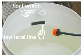
Low level line and float switch
