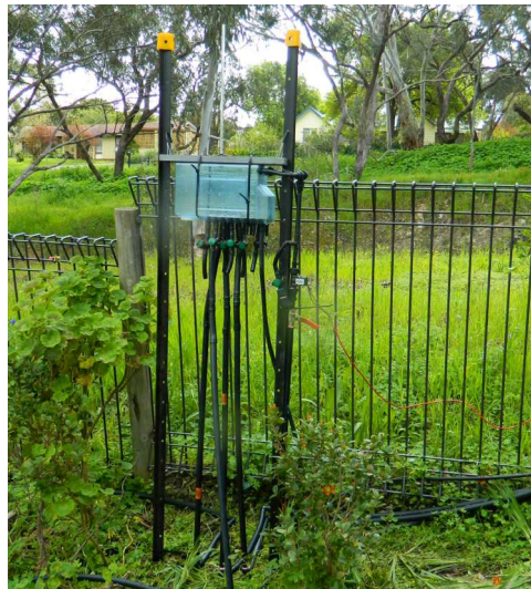
Flow-splitter mounted on star pickets
