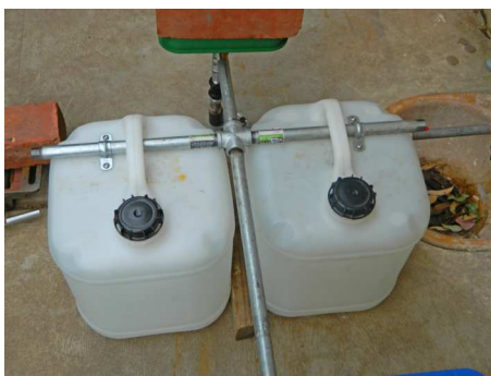
Secure the pivot points with two 20 litre water containers
