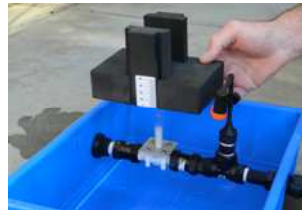
Slide the float over the float shaft
