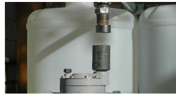
When the rare earth disc magnet assembly is in the high position, the top of the solenoid should be 20mm below the magnet
