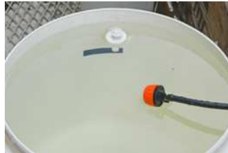
Irrigation stops when the water level reaches the float switch,
