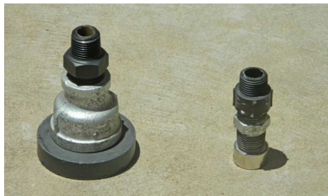
Ferrite ring magnet assembly on the left Rare earth disc magnet assembly on the right
