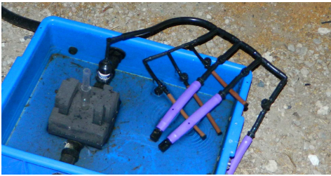
Precision adjustable dripper with 3 Netafim Miniscape drippers and 3 Netafim Bioline drippers.
