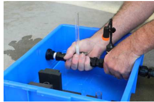
Float shaft must be vertical
