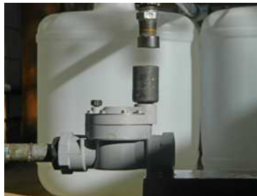
When the magnet is in the high position, the plunger is released and the valve closes
