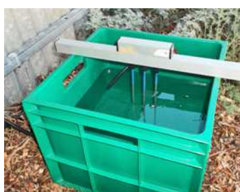
Evaporator and level sensor with 3 probes
