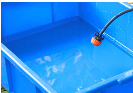
Position the adjustable dripper so that it will drip water into the evaporator
