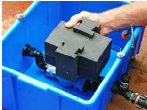
Position the float over the solenoid
