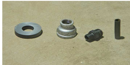
Components of the ferrite ring magnet assembly
