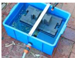
13mm net evaporation between irrigation events (zero gap between magnet and bottom of full slides)
