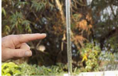
The pressure monitor tube shows a pressure of about a metre head of water
