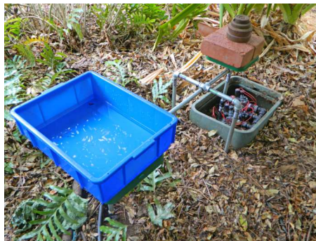
Add water to the evaporator until the depth is a least 20mm
