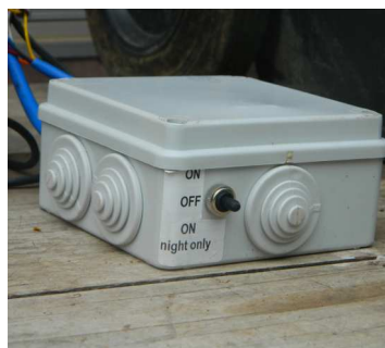
The switch on the irrigation controller has 3 positions
