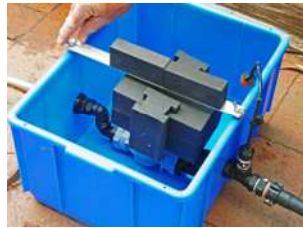
Use the two wing-nuts to secure the aluminium bar
