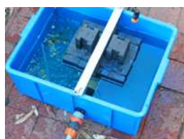
19mm net evaporation between irrigation events (zero gap between magnet and bottom of full slides)
