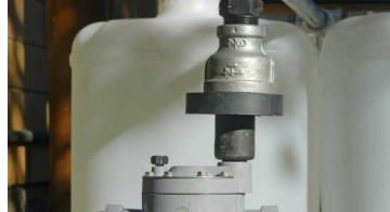
When the ferrite ring magnet assembly is in the high position, the top of the solenoid should be 10mm inside the ring magnet
