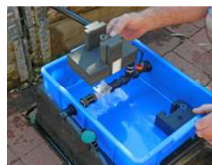
Slide the float over the float shaft
