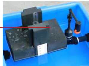
The irrigation stops when the float reaches the high level
