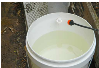
While the soil is drying, the water level in the evaporator is falling due to evaporation
