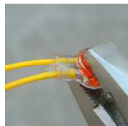
Gel is squeezed out of connector
