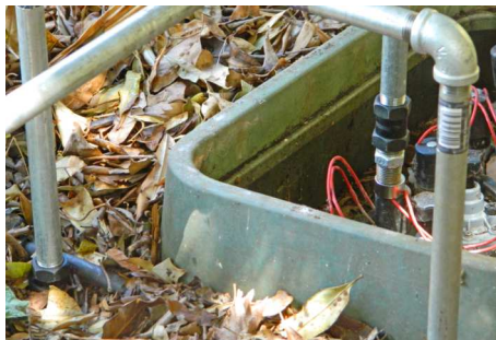
Water slowly evaporates from the evaporator until the weight of the water in the evaporator is light enough for the magnet to fall from the high position to the low position
