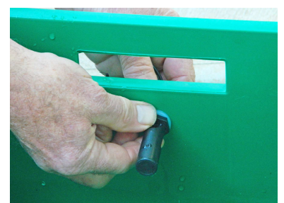
Install the float switch
