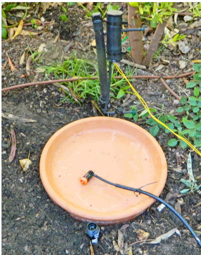
In ground installation of the Large Terracotta Irrigation Controller for Latching Solenoids
