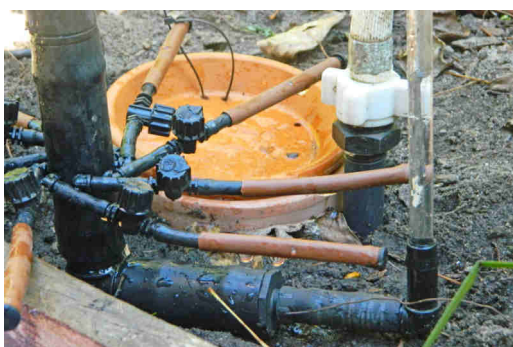
Fraction 2/7 for 8mm Netafim dripline (1 closed lower dripper, 7 open lower drippers and 2 open lower drippers as control dripper) water supply pressure 100 kPa. This setup is used for a garden in Adelaide with more than 400 drippers.
