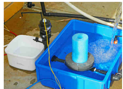
Fill the evaporator with water until the water stops flowing from the two outlets
