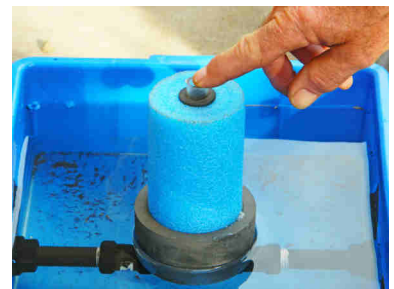
Push the float down to start irrigating
