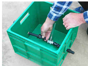
Insert the outlet pipe through the other hole
