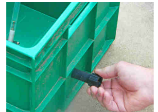
Attach a round plastic nut
