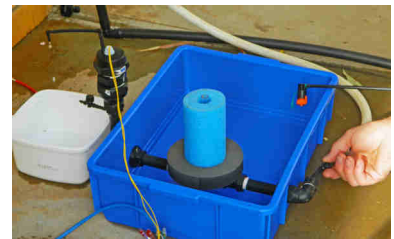
Close the small valve connected to the water supply until water drips at about 6 drips per second
