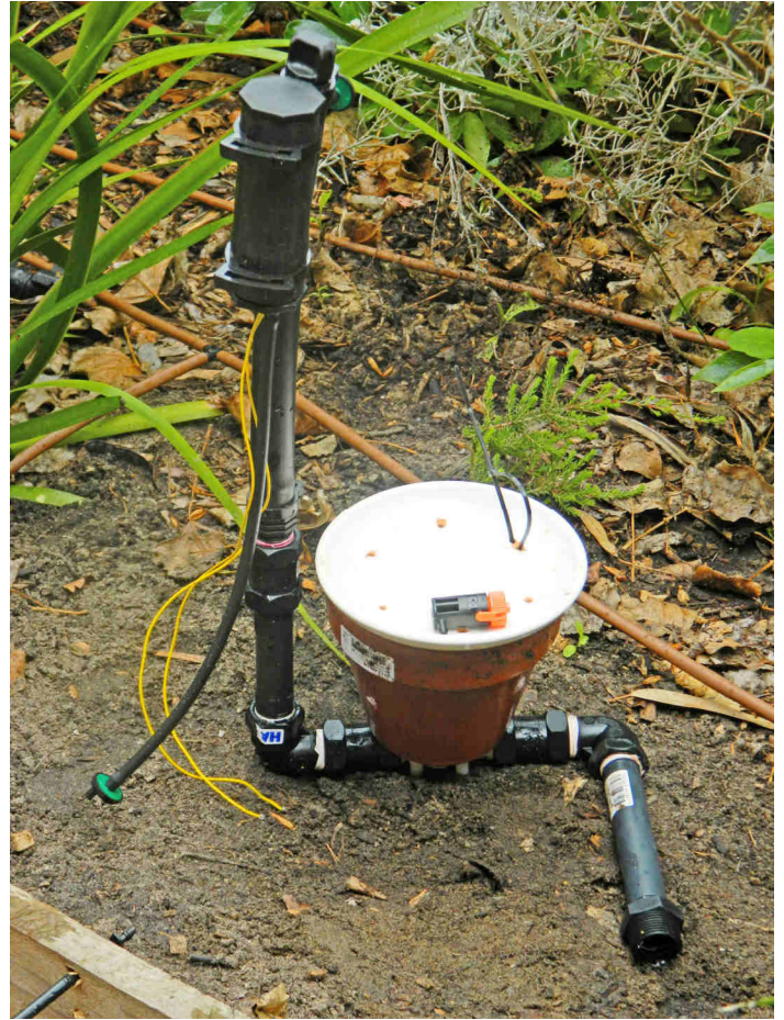
Above ground installation of the Terracotta Irrigation Controller for Latching Solenoids
