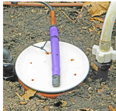
The adjustable control dripper has been replaced by an in-line irrigation dripper.
