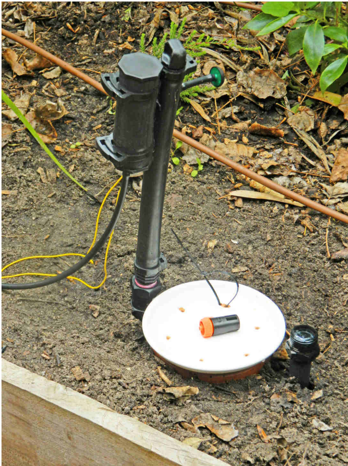
In ground installation of the Terracotta Irrigation Controller for Latching Solenoids
