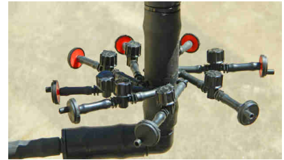
Each of the lower drippers is connected to a 4mm micro valve
