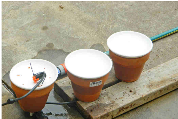
With two additional pots the discharge during the irrigation event is slightly more than trebled.
