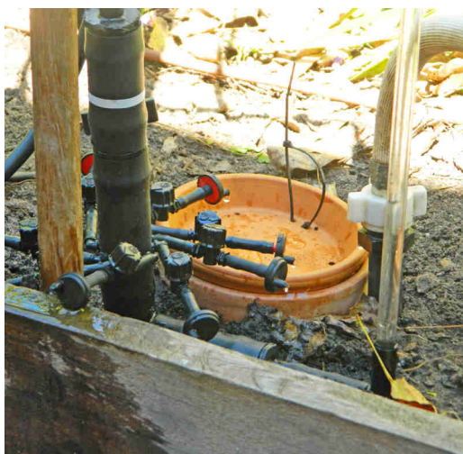
Fraction 1/8 for online drippers (8 open lower drippers, one lower dripper as control dripper) water supply pressure 40 kPa
