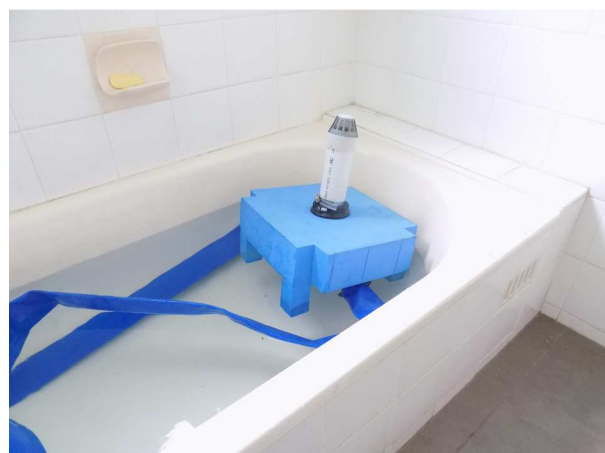
the float valve rises and falls according to the water level in the pond
