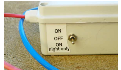
Switch with 3 positions: ON, OFF, ON night only
