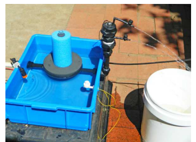
When the float reaches the high level the irrigation stops
