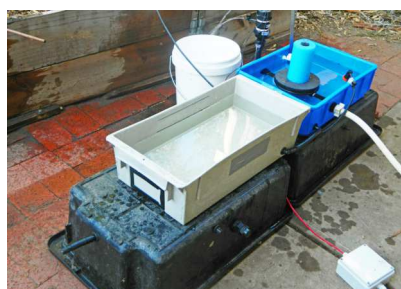
A supplementary evaporator increases the surface area of evaporation
