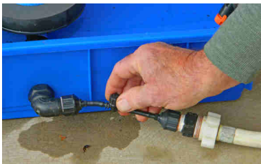
Close the small valve on the side of the evaporator
