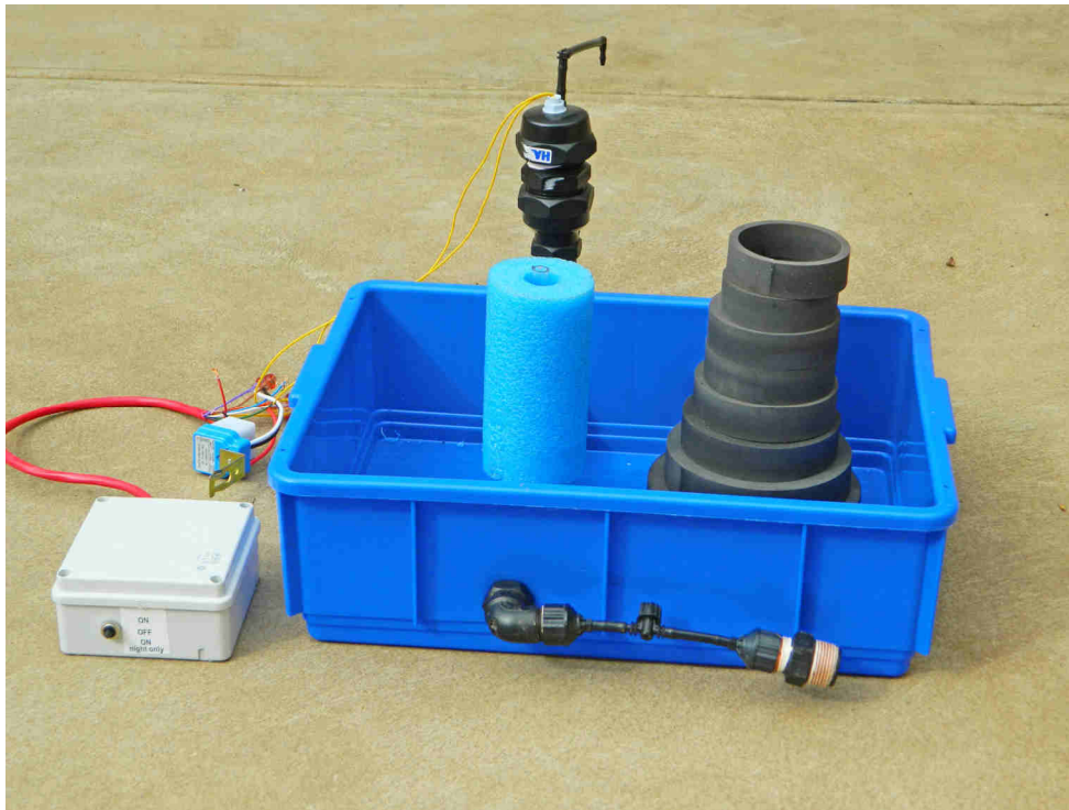
Universal Measured Irrigation Controller components
