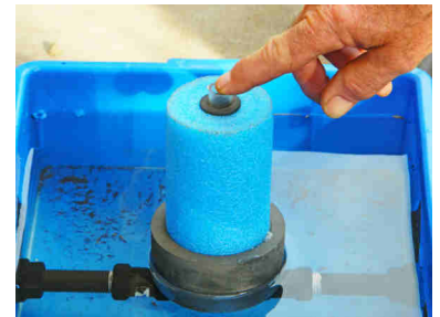
Push the float down to start irrigating
