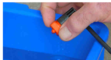
Turn the control dripper to change the flow rate
