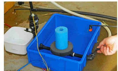
Open the small valve connected to the water supply until water drips at about 6 drips per second
