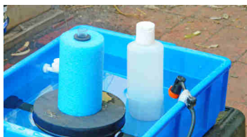
A full bottle of water decreases the surface area of evaporation
