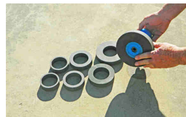
Float cylinder and 7 float rings
