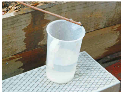
Dripper control volume for root zone scheduling
