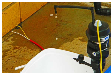
Water dripping from the top outlet at about 6 drips per second
