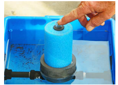
Push the float down to start irrigating
