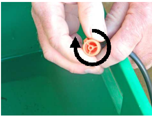
Turn the control dripper clockwise to reduce the flow rate
