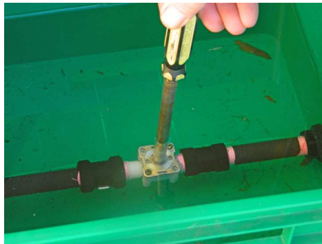
To adjust the irrigation frequency turn the control screw anticlockwise the desired number of turns
