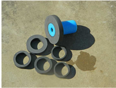
Cylindrical float and six float rings
