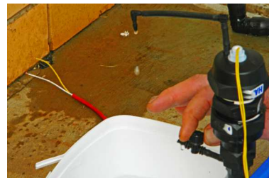
Slowly open the small valve connected to side of the vertical tube until water is dripping from both outlets at the same rate
