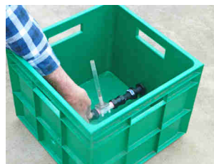
Insert the inlet pipe through one of the holes
