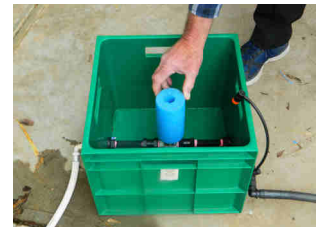
Slide the cylindrical float over the float shaft
