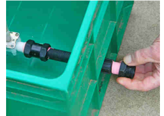
Attach the inlet adaptor to the inlet pipe
