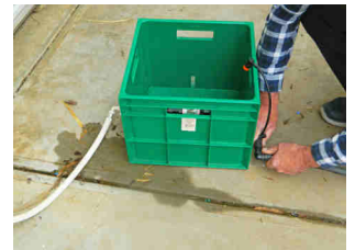
Connect the irrigation system to the outlet side of the evaporator
