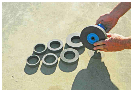
Slide the float ring over the cylindrical float
