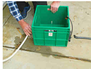
Connect the water supply to the inlet side of the evaporator
