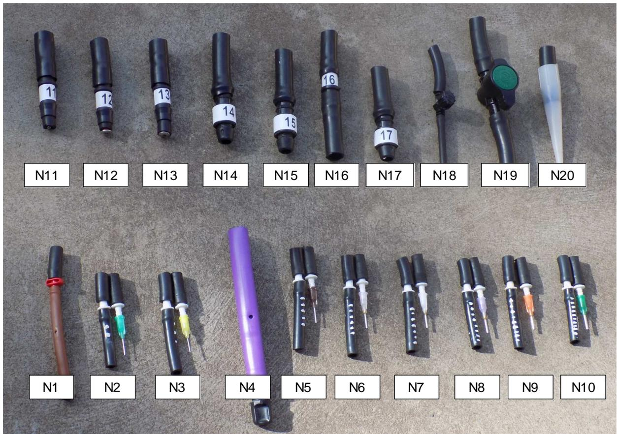
Nozzles available from the measured irrigation website (flow-splitter nozzles illustrated). The needle nozzles are illustrated both with and without the protective black tube.
