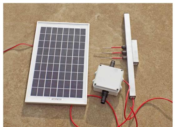
Solar-powered automated single-zone measured irrigation kit: solar panel, solenoid valve and level sensor
