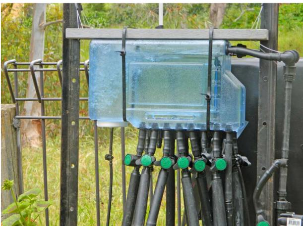
In the photo on the left a tube is connected to the control nozzle. This tube delivers water to the evaporator. The irrigation event will stop when the control volume of water has been delivered to the evaporator. The other tubes are delivering water to the various irrigation zones
