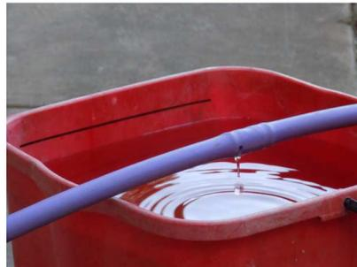
A pressure compensating dripper drips water into a bucket.
