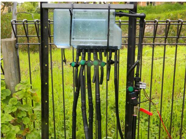
Flow-splitter variable nozzles and the control nozzle on the right
