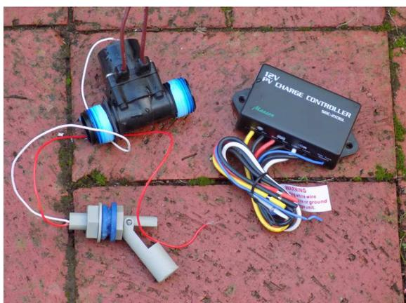
Float switch, solenoid valve and charge controller 36 -
