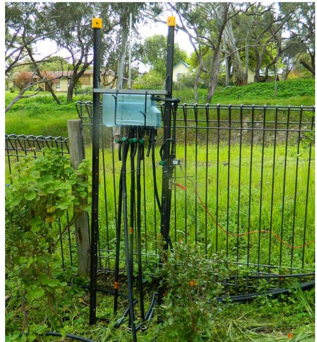
Flow-splitter mounted on star pickets
