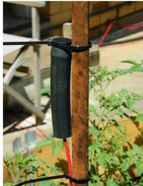
One way of protecting the relay from the weather is to house the relay in a short length of vertical polypipe with a plug at the top.
