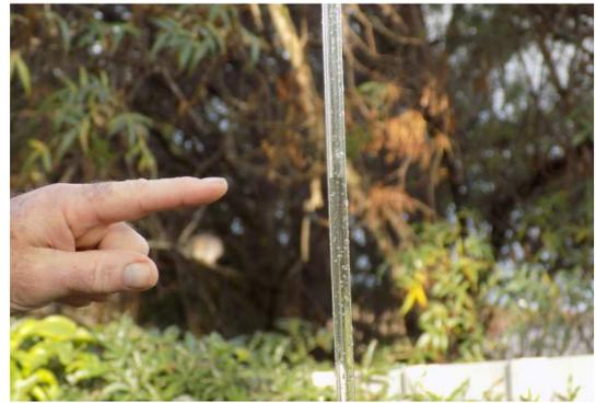
The pressure monitor tube shows a pressure of about a metre head of water
