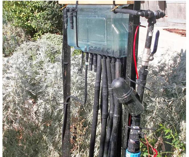
Flow-splitter measuring the water delivered to each of the eleven irrigation zones
