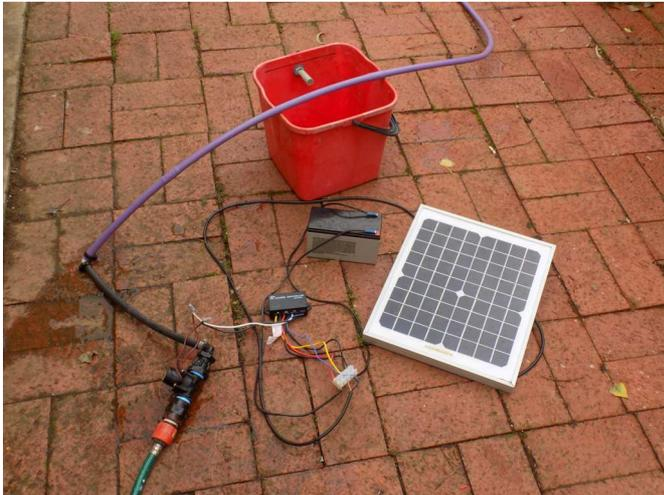
Solar panel, battery, charge controller, solenoid valve and float switch
