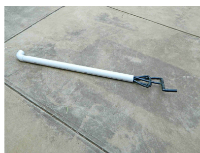
The dripper assembly is inserted inside an open pipe and is ready to be connected to the 25 mm polypipe.
