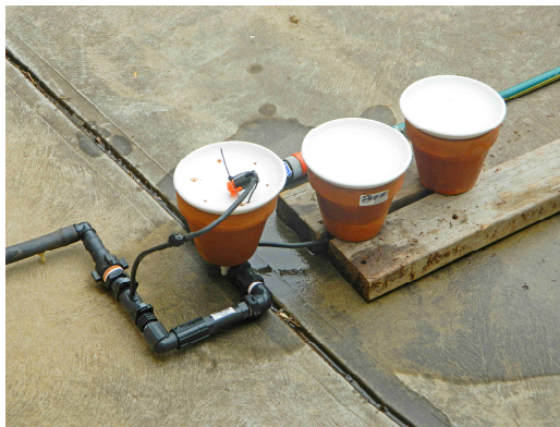
With two additional pots the discharge during the irrigation event is slightly more than trebled.
