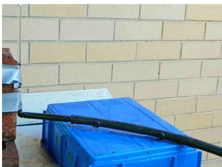
Zone 1 with 2 drippers at level -1.74 metres.
