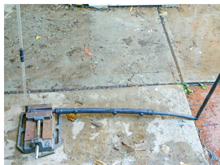
Zone 2 with 3 drippers at level -2.77 metres.
