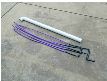
Dripper assembly for zone 8 with 15 8 L/H drippers using Netafim Aries HWD 13 mm dripline
