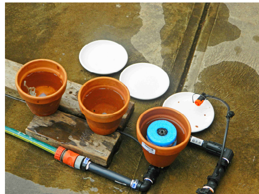
The pots are connected by 4 mm tubing so that the water level is the same in all the pots.
