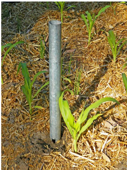
The steel pipe is hammered into the soil near a dripper.
