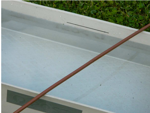
One of the MI drippers drips water into the evaporator during the irrigation event.
