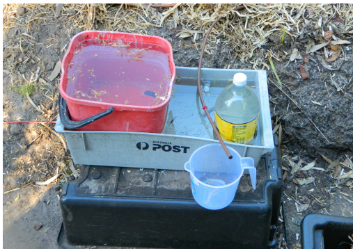
The volume of water emitted by a MI dripper is measured by collecting the emitted water in a measuring cup as shown.
